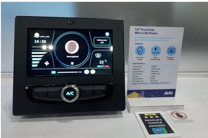
A 1" true-circle automotive microLED display prototype, with an embedded fingerprint sensor (AUO)
