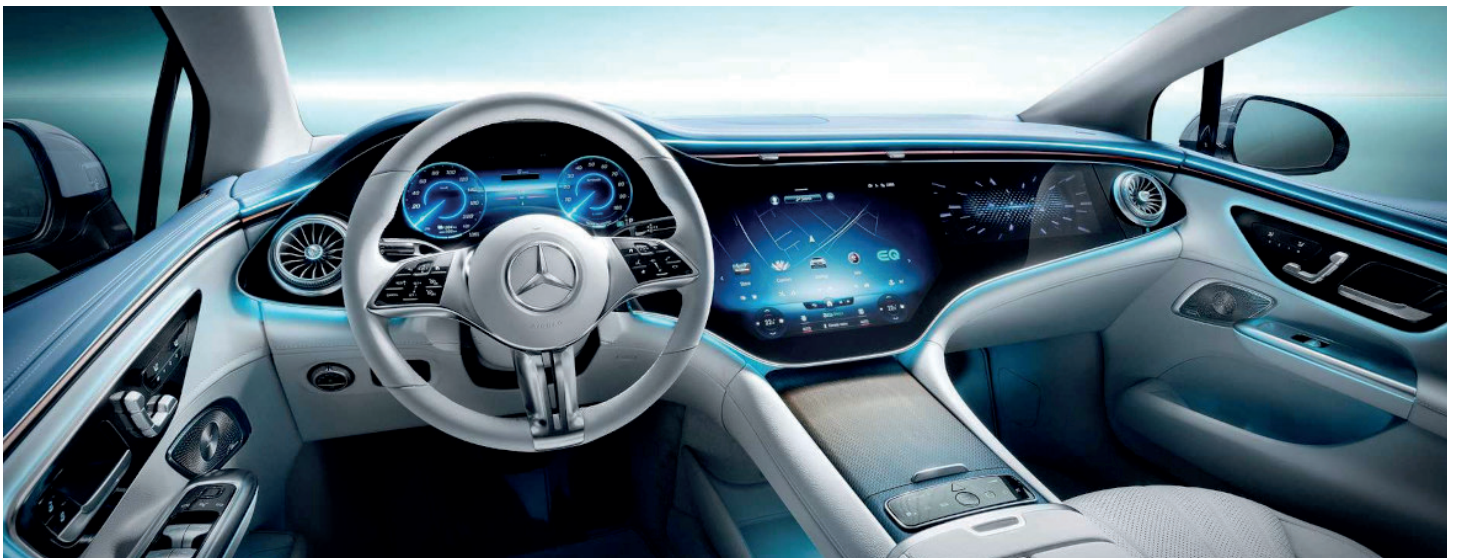
The 2022 Mercedes EQE EV, with the 56" MBUX OLED Hyperscreen (3 OLED panels under a 56-inch glass, produced by LG Display)
